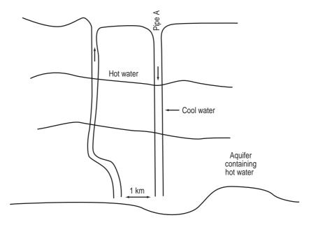
Figure 1.13: How to tap geothermal energy
