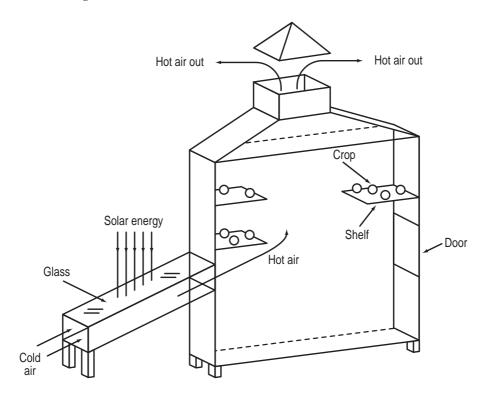
Figure 1.12: An indirect solar drier. This device is used to dry valuable crops.
